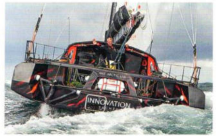
Opposite: with a dry ship displacement of 9.5 tonnes Norbert Sedlacek's 'sailing volcano' is at least 1,500kg heavier than a current Imoca of the same length, but the extra weight is primarily down to the reinforcement required for a yacht that will bounce off the ice floes of the Northwest Passage... along with the structure for 73 flotation compartments. Another slice of additional weight is down to the materials used, with a core (below) of sustainable balsa replacing the Nomex in all today's Imocas. The resin used is also recyclable. The construction matrix was trialled in the 16ft Fipofix (above left) which has now completed two solo atlantic crossings...
