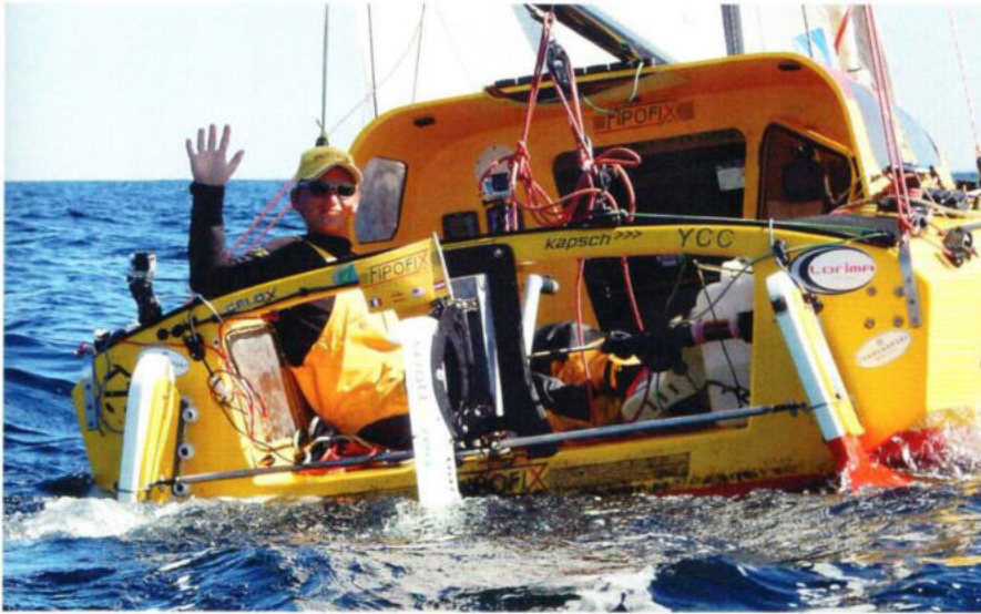
Opposite: with a dry ship displacement of 9.5 tonnes Norbert Sedlacek's 'sailing volcano' is at least 1,500kg heavier than a current Imoca of the same length, but the extra weight is primarily down to the reinforcement required for a yacht that will bounce off the ice floes of the Northwest Passage... along with the structure for 73 flotation compartments. Another slice of additional weight is down to the materials used, with a core (below) of sustainable balsa replacing the Nomex in all today's Imocas. The resin used is also recyclable. The construction matrix was trialled in the 16ft Fipofix (above left) which has now completed two solo atlantic crossings...
