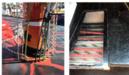
All lines are led aft under deck or in tunnels to prevent icing up. The line tunnels also provide extra structure.
