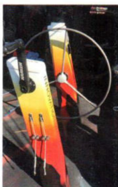
Sedlacek has a single wheel protected under the coachroof – with two back-up tillers – and a pedestal winch in the cockpit.
