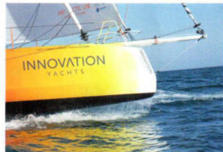
The entire bow area is reinforced monolithic construction for nudging ice out of the way.
