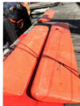
There are three boards, two interchangeable daggerboards and one central canard to protect the keel fin.
